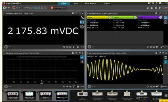
Figure 4. View measurements across USB DAQ, modular, and bench instruments all on one BenchVue interface.
